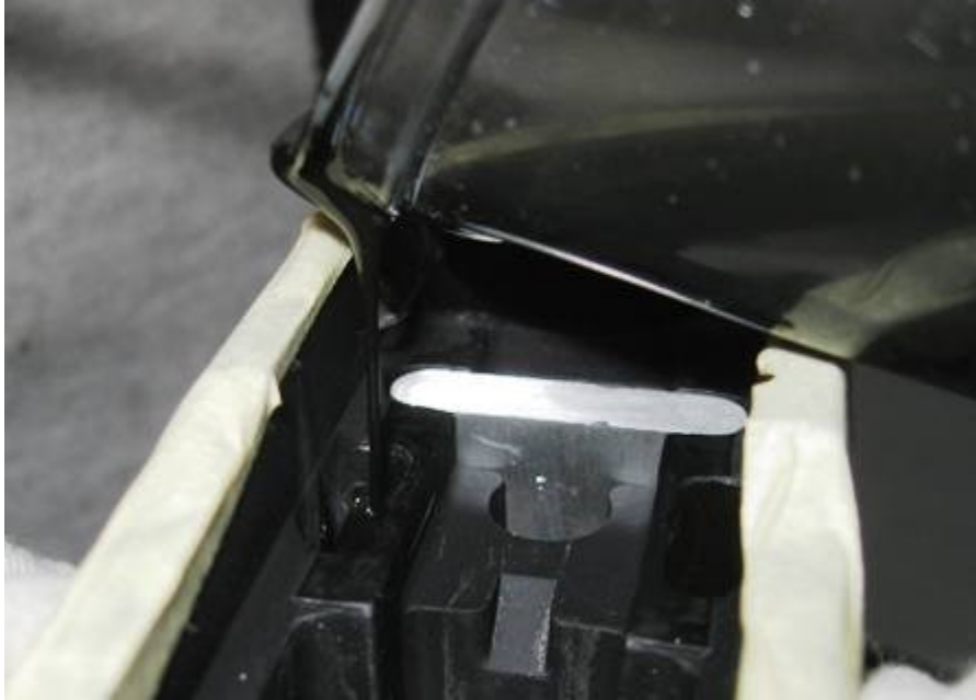
Filling skeletal voids within the action area of a Sako A7 stock.
