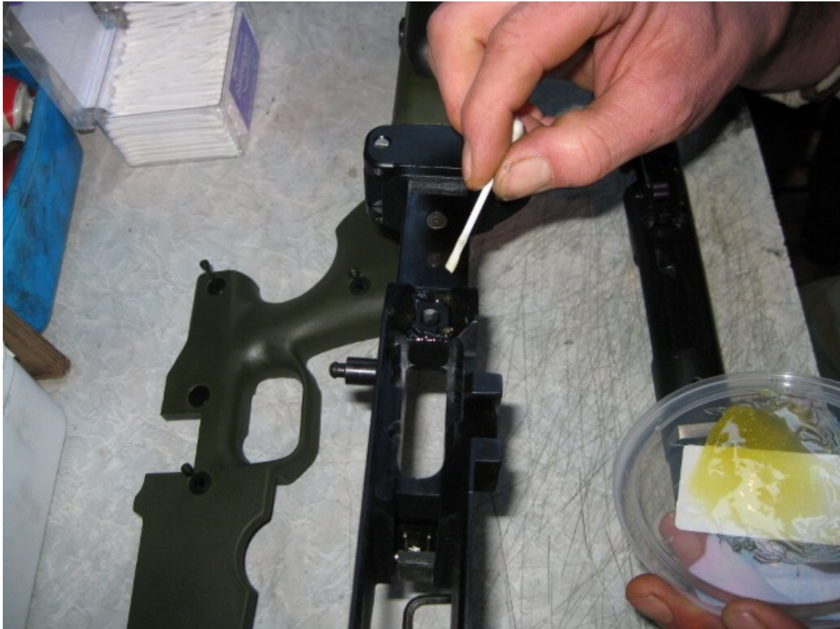
An Accuracy International stock, plastic panels removed. In this photo, I am applying a basic two pot (double syringe) epoxy to the V block at the tang prior to rigid mounting
