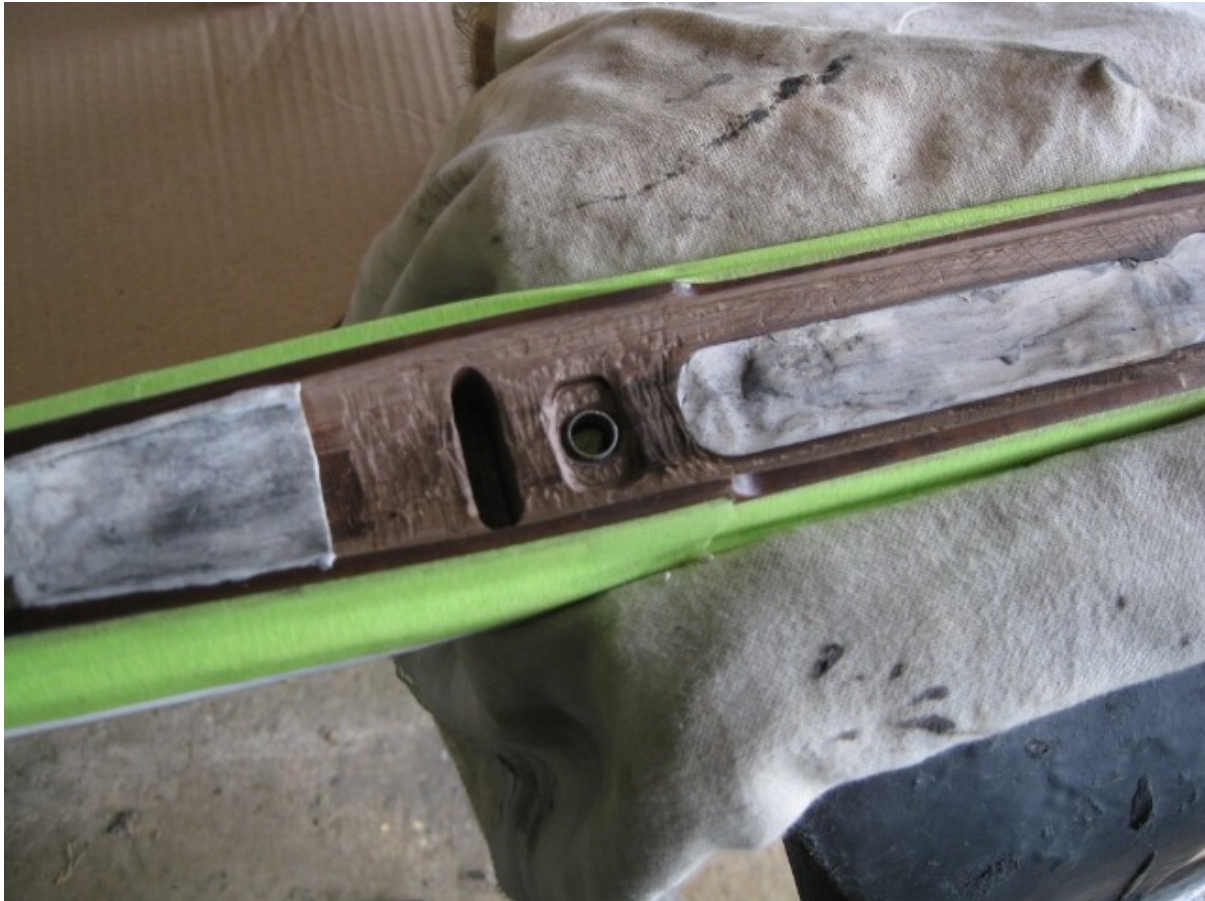
Tikka rifle stock showing front steel pillar inserted during the bedding process. Heavy walled aluminum pillars (wide diameter) are also common.
