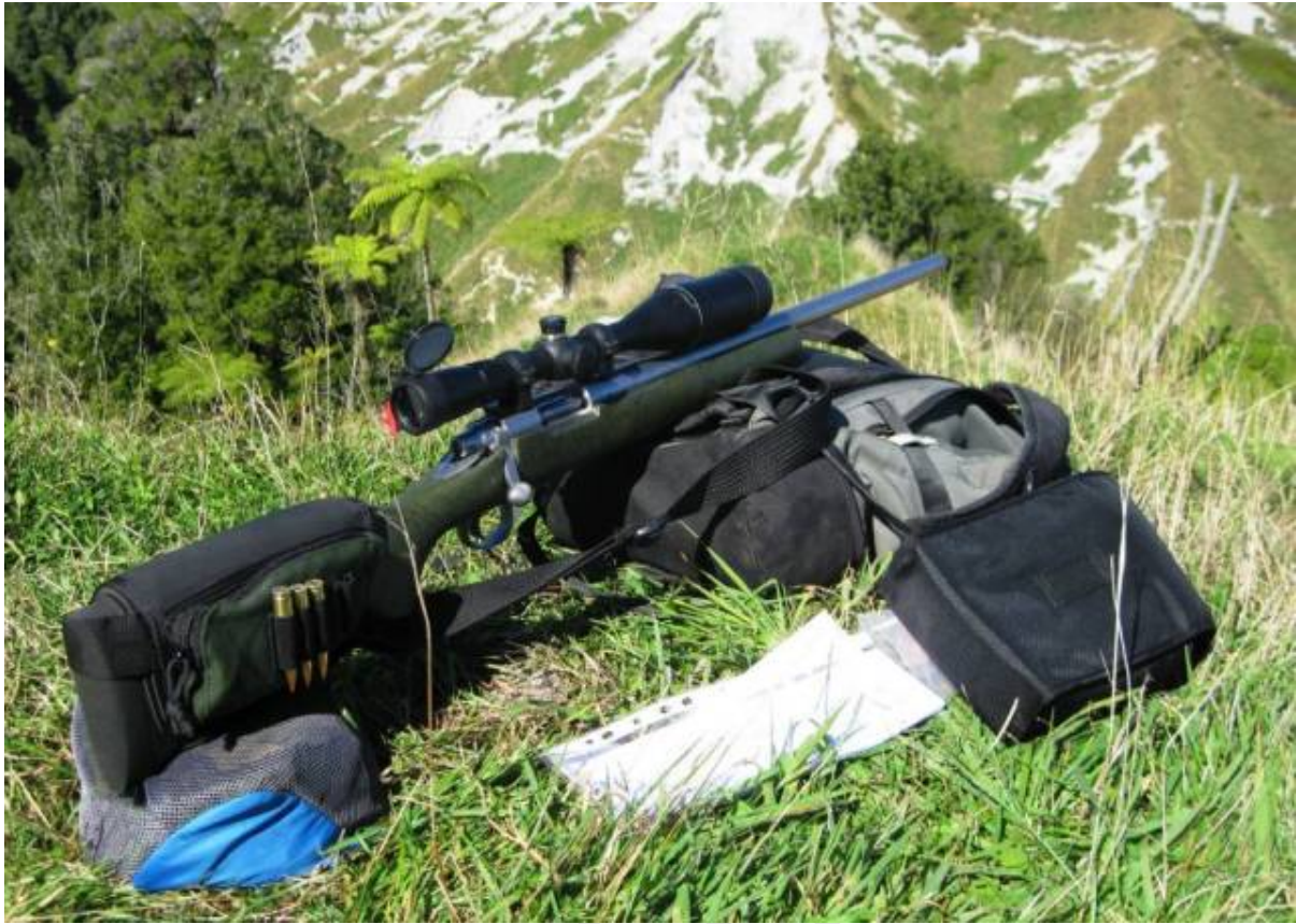
Remington 5R .308 Winchester. This rifle is wearing a Bell and Carlson #2958 stock. Note the cheek wallet attached to the butt of the rifle, used to raise the height of the comb.
