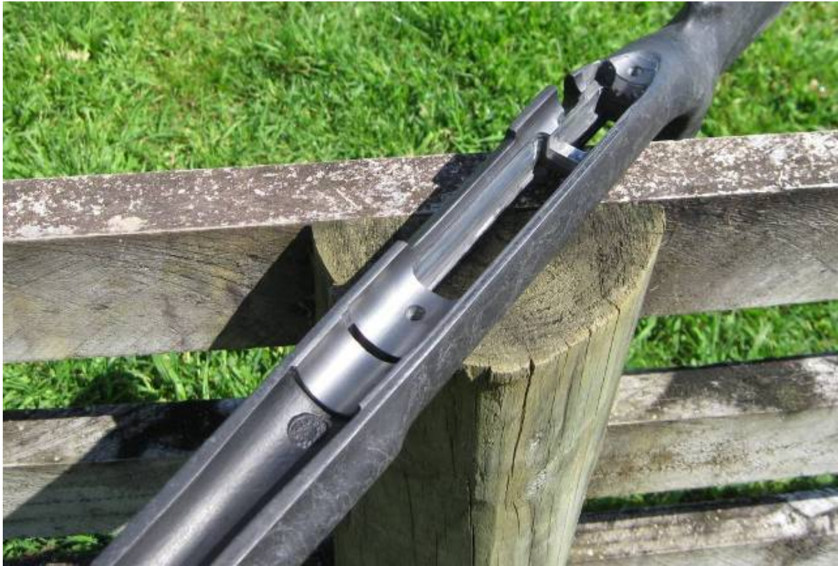
The HS stock, bedded with our MatchGrade steel based bedding compound.
